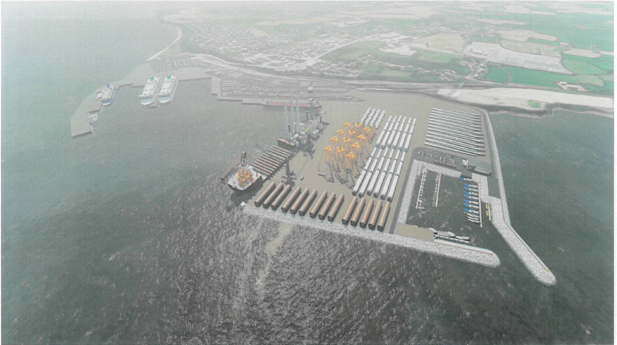
Figure 3-4: Example of operational layout including turbine tower and foundation vessel loading operations quayside (aerial view seaward side)
