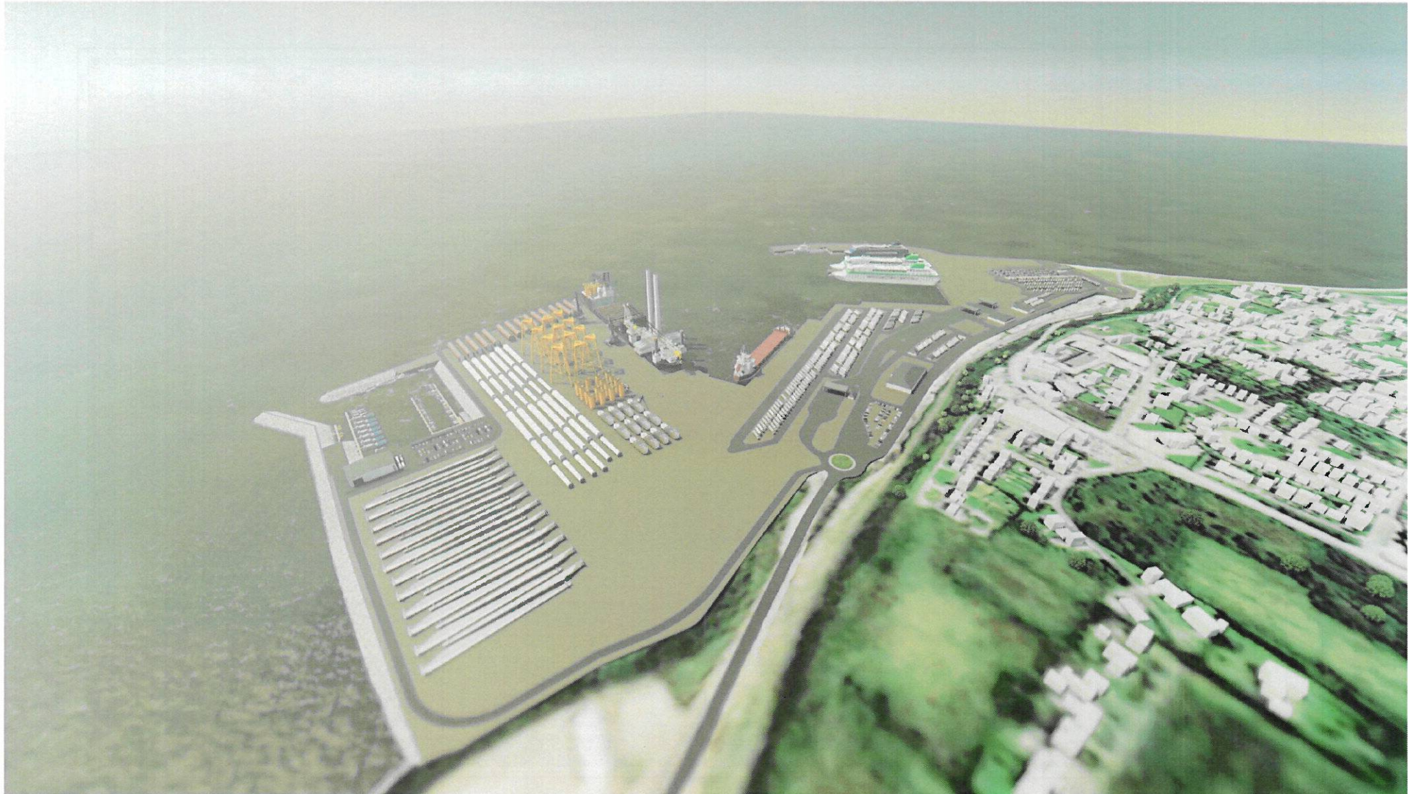
Figure 3-3: Example of operational layout including turbine tower and foundation vessel loading operations quayside (aerial view from land)
